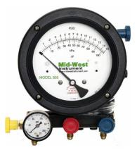
Many testers find it more convenient to hold the test kit from the bottom, sometimes inadvertently covering the low side hose connection with the palm of their hand. This situation prevents the diaphragm from moving properly. Once the diaphragm is no longer allowed to "breath" as the pressure decreases on the high side, a vacuum is created preventing the needle on the gauge to drop sufficiently to
